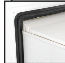
Sliding a room in and out poses some out-of-the-way engineering and sealing challenges to do it right. Newmar developed an improved slideout wedge roof design that forms a tighter closure when the room is extended. A specially developed double-bulb, superior-memory seal provides protection from outside elements and insects, and sweeps off debris on room retraction.
