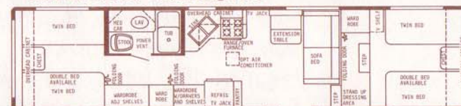
35' Center Bath - Dry Wt. 8500 lbs. - Hitch Wt. 1650 lbs. - Overall Length 35'6"
