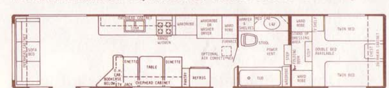
40' Walk-Thru Front Bath 2-Door - Dry Wt. 9300 lbs. - Hitch Wt. 1650 lbs. - Overall Length 39'6"
