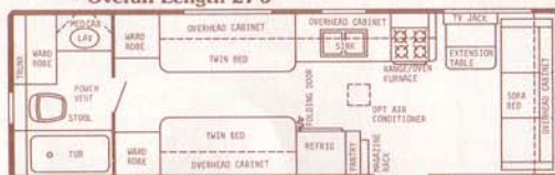
29' Rear Bath - Dry Wt. 6500 lbs. - Hitch Wt. 675 lbs. - Overall Length 29'5"
