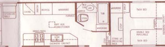
35' Walk-Thru Front Bath 2-Door - Dry Wt. 7500 lbs. - Hitch Wt. 1750 lbs. - Overall Length 32'6"
